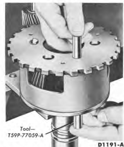
FIG. 18—Long Pinion Removal or Installation
