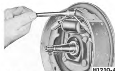
FIG. 5—Retracting Spring Removal
