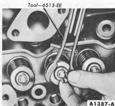
FIG. 29—Compressing Valve Spring
