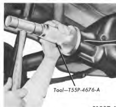
FIG. 16—Drive Pinion Flange Seal Installation
