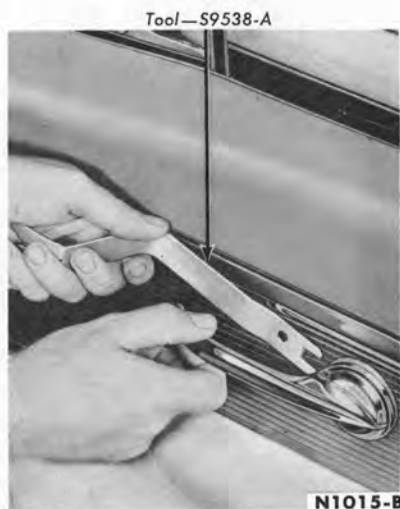
FIG. 8—Typical Handle Removal
