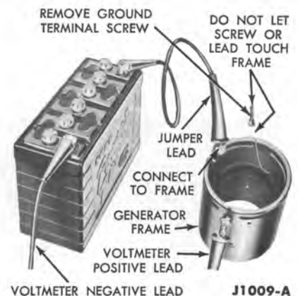
FIG. 7—Field Grounded Circuit Test
