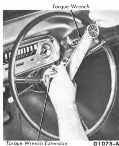
FIG. 2—Steering Gear Load Check
