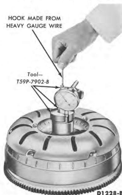
FIG. 2—Turbine and Stator End Play Check
