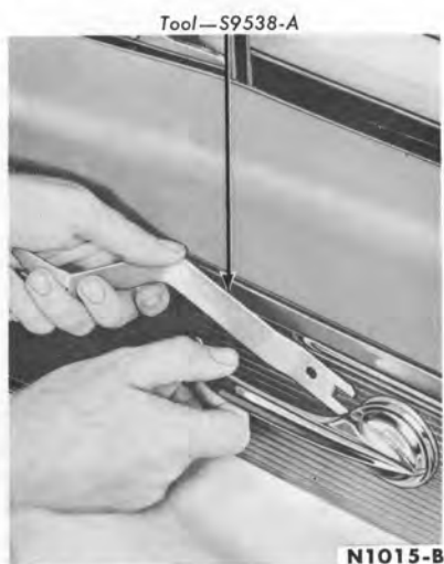
FIG. 4—Typical Inside Door Handle Removal
