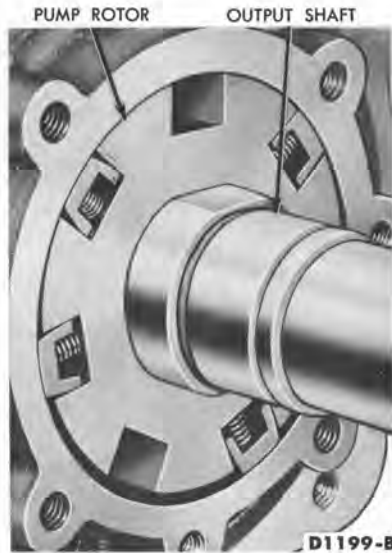
FIG. 25—Rear Pump Rotor Alignment
