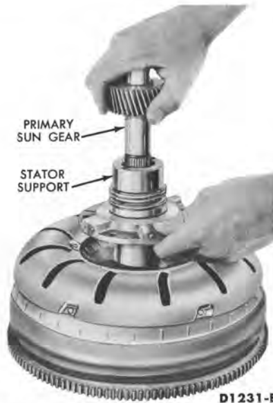
FIG. 5—Stator to Turbine Interference Check
