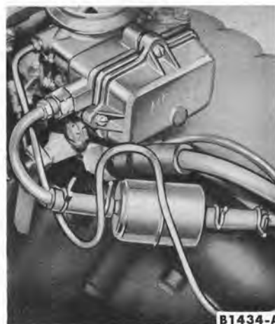
FIG. 5—Fuel Filter Installation—Typical
