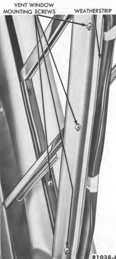
FIG. 11—Vent Window Installed
