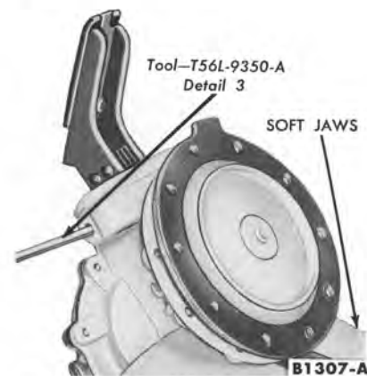
FIG. 1—Rocker Arm Pin Removal or Installation
