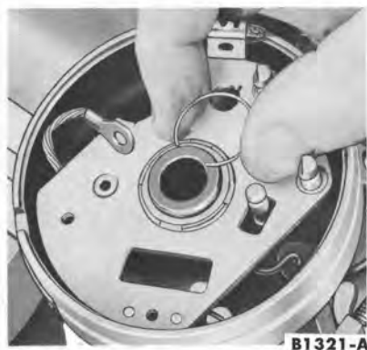
FIG. 12—Lock Ring Installation
