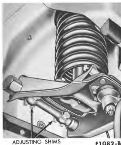
FIG. 2—Upper Arm Assembly
