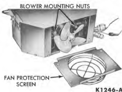
FIG. 16—Blower Motor Mounting
