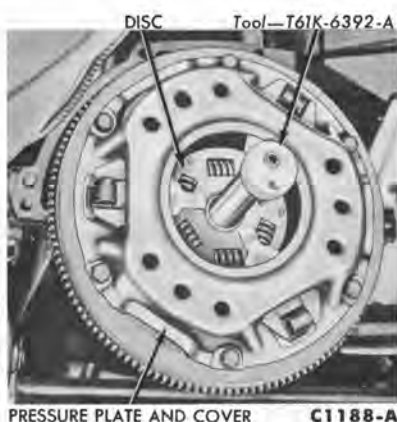
FIG. 8—Disc Alignment
