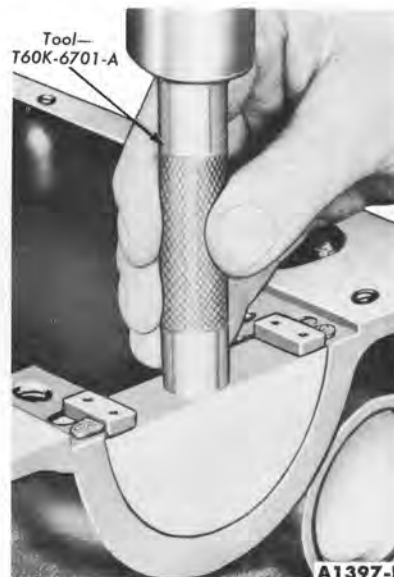
FIG. 73—Rear Oil Seal To Block Installation
