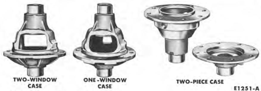
FIG. 2—Falcon Differential Cases
