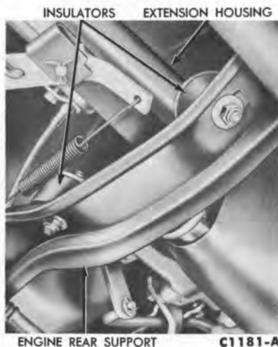
FIG. 4—1960 and Early 1961 Extension Housing Mounting—Station Wagon
