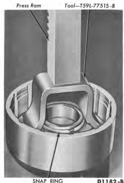
FIG. 11—Clutch Spring Snap Ring Removal
