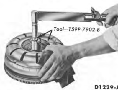
FIG. 3—Stator One-Way Clutch Check
