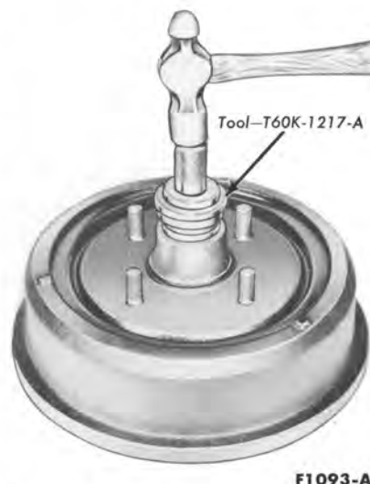
FIG. 6—Front Wheel Bearing Cup Installation
