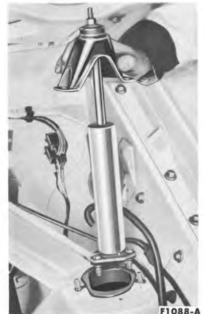
FIG. 9—Front Shock Absorber Removal
