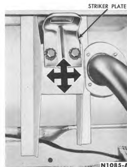
FIG. 37—Deck Lid Striker Plate Adjustment
