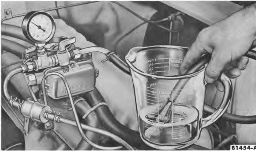
FIG. 2—Fuel Pump Pressure and Capacity Test—Typical
