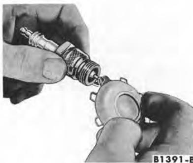
FIG. 18—Gapping Spark Plug
