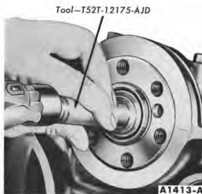
FIG. 83—Clutch Pilot Bushing Installation
