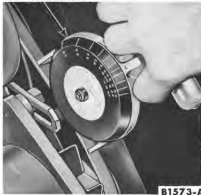
FIG. 2—Drive Belt Tension Adjustment
