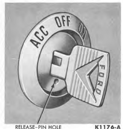
FIG. 10—Ignition Switch Removal
