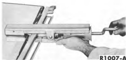
FIG. 10—Glass Channel Replacement
