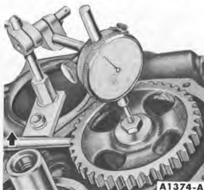
FIG. 51—Camshaft End Play
