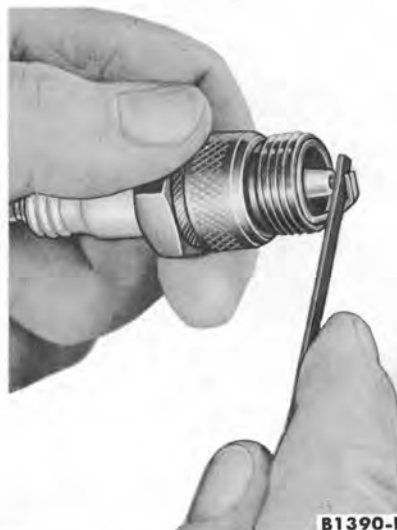
FIG. 17—Cleaning Plug Electrode
