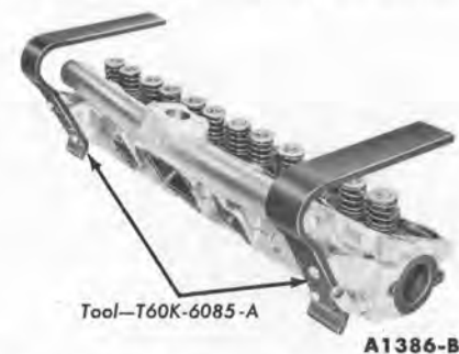
FIG. 28—Cylinder Head Holding Fixtures
