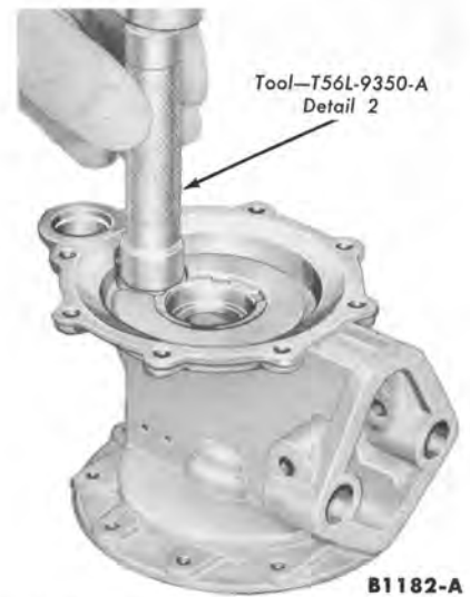
FIG. 4—Booster Pump Valves and Gaskets Installation
