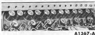
FIG. 25—Valve Push Rod Removal
