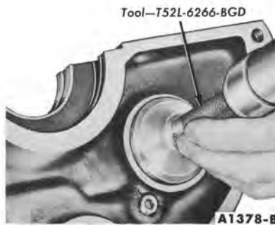
FIG. 79—Camshaft Rear Bore Plug Installation
