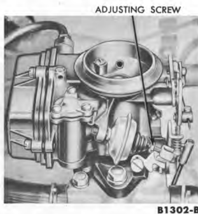
FIG. 9—Anti-Stall Dashpot Adjustment—1960 and 1961 Models
