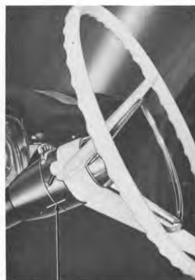
FIG. 1 — Straight-Ahead Position Marks
