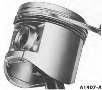
FIG. 65—Ring Side Clearance
