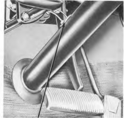
FIG. 5—Starter Neutral Switch
