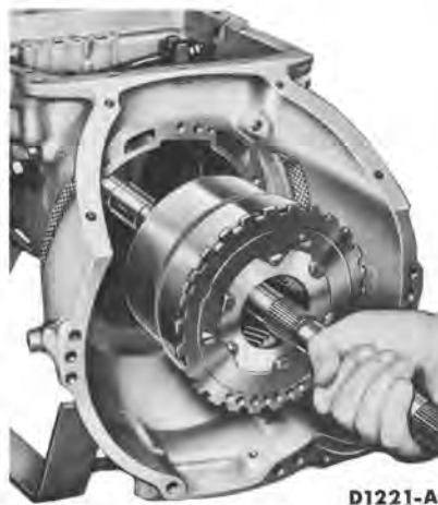
FIG. 4—Output Shaft Removal or Installation
