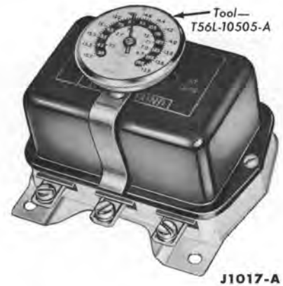
FIG. 13—Voltage Regulator Setting Thermometer
