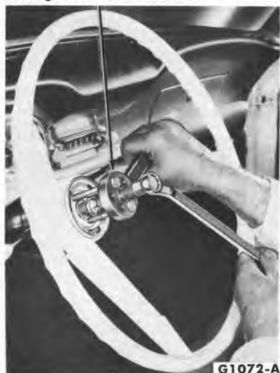
FIG. 4—Steering Wheel Removal
