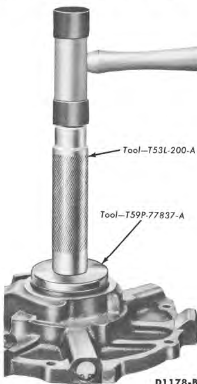
FIG. 7—Front Pump Seal Installation
