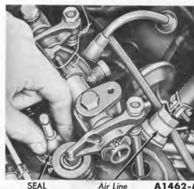
FIG. 44—Valve Stem Seal Removal
