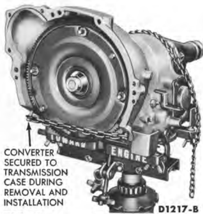
FIG. 4—Transmission Mounted in Jack
