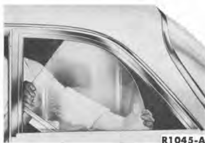
FIG. 18—Quarter Window Glass Removal
