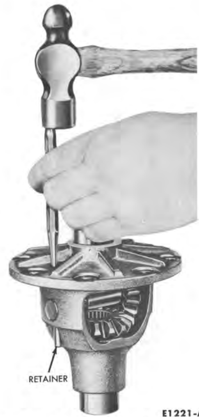
FIG. 14—Differential Pinion Shaft Retainer Removal
