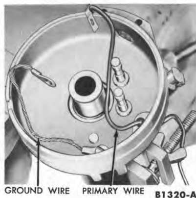
FIG. 11—Primary and Ground Wire Installation
