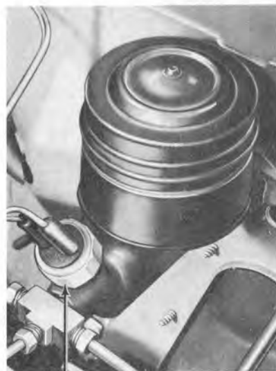
FIG. 8—Stop Light Switch
