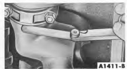
FIG. 56—Connecting Rod Side Clearance
