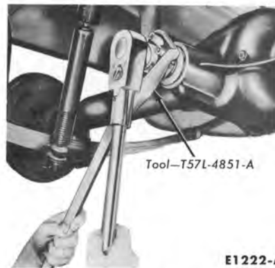
FIG. 9—Drive Pinion Shaft Nut Removal
