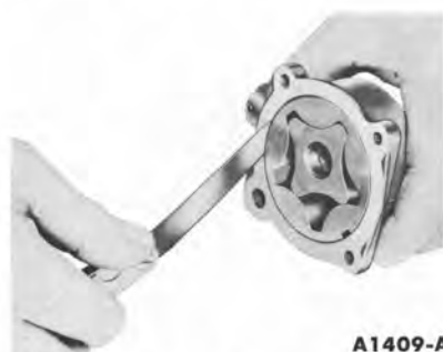
FIG. 69—Outer Race To Housing Clearance
