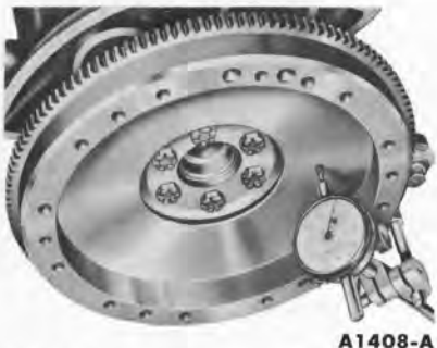
FIG. 66—Flywheel Face Runout
