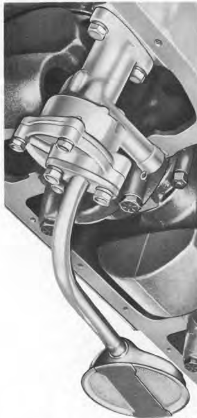
FIG. 68—Oil Pump Inlet Tube Installed
