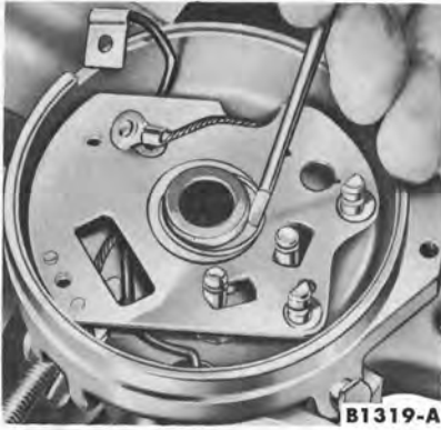
FIG. 6—Lock Ring Removal
