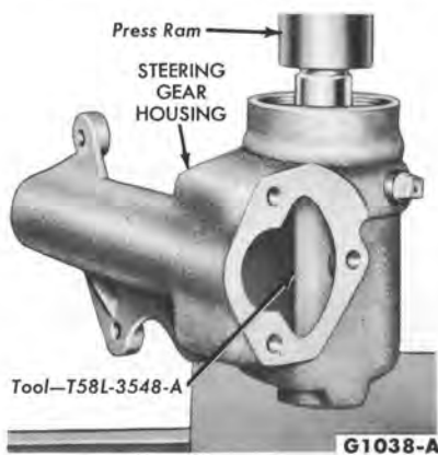
FIG. 9—Steering Shaft Lower Bearing Cup Installation
