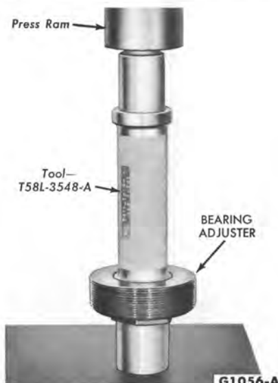
FIG. 10—Steering Shaft Upper Bearing Cup Installation
