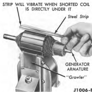
FIG. 4—Growler Test for Shorted Armature
