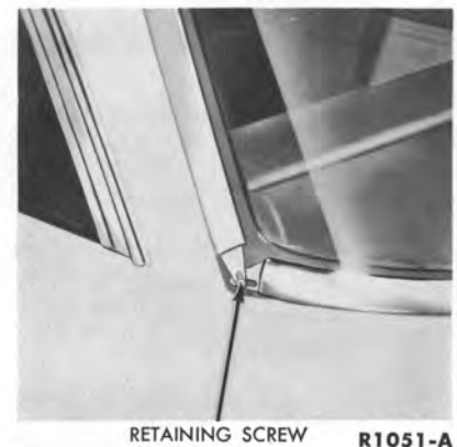
FIG. 25—Back Window Outside Moulding Screw
