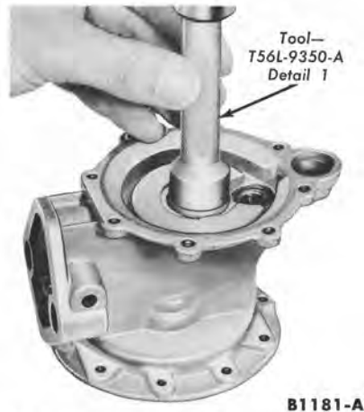
FIG. 3—Diaphragm Rod Oil Seal and Retainer Installation
