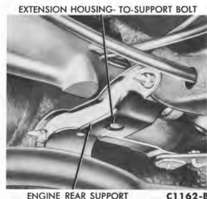
FIG. 5—1960 and Early 1961 Extension Housing Mounting—Sedan
