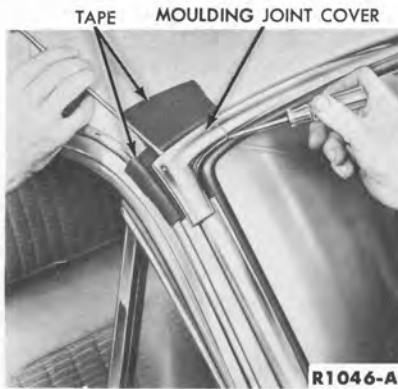
FIG. 21—Moulding Joint Cover Removal
