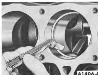
FIG. 64—Piston Ring Gap
