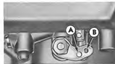
ACCELERATION PUMP STROKE SUMMER— PUT ROD IN HOLE A WINTER— PUT ROD IN HOLE B B1578-A
