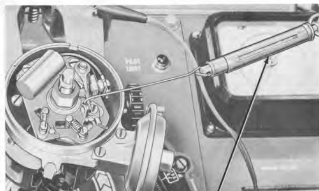
FIG. 13—Checking Breaker Point Spring Tension
