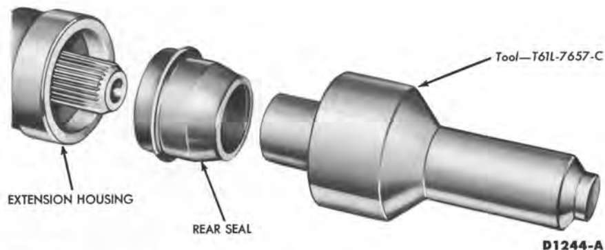
FIG. 3—Extension Housing Seal Installation
