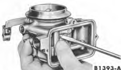
FIG. 11—Main Well Body Installation—Typical
