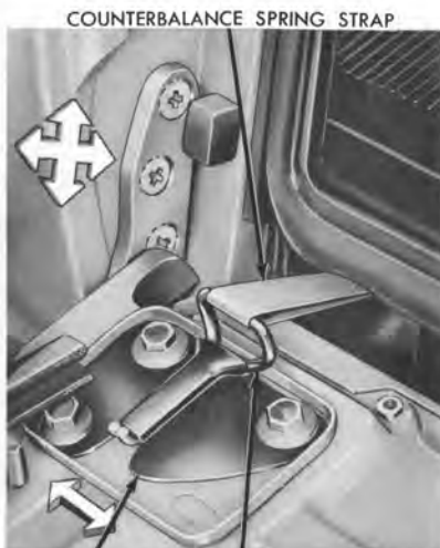
FIG. 32—Tailgate Hinge Adjustment
