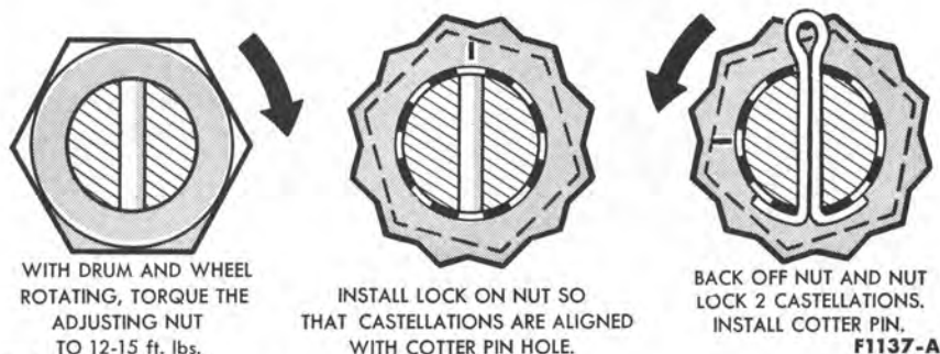
FIG. 5—Front Wheel Bearing Adjustment
