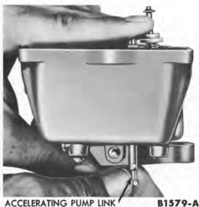
FIG. 23—Accelerating Pump Link Removal or Installation
